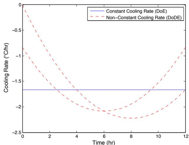
Fig. 1. Examples of possible cooling rates using the DoE and DoDE methodologies. DoE can only evaluate constant cooling rates whereas DoDE can evaluate any constant or non-constant cooling rate profile.
