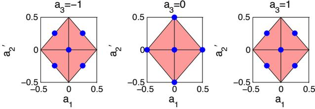
Fig. 5. Graphical representation of experimental points for the central composite design ( $a_2' = a_2 + 0.5$ ).
