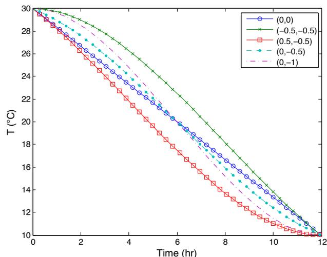
Fig. 3. Temperature profiles for different values of  $(a_1, a_2)$  inside the design space. All profiles meet the constraints set by (2)-(4). The linear cooling profile (constant cooling rate) is marked with open circles for reference.
