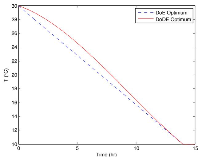
Fig. 7. Optimum cooling profiles from the DoE and DoDE designs. The DoDE method is able to determine optimum nonlinear cooling trajectories.
